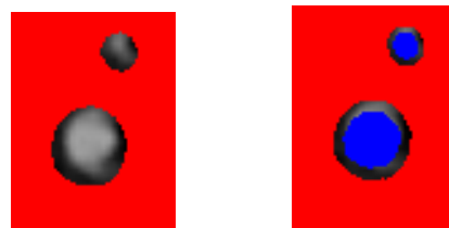
Fig. 9. (Left) A tubular structure extracted from a 3D volume. (Right) A tubular structure containing an interior radius defining a hollow region (the blue segment.) We do not extract the voxels contained within this region.
