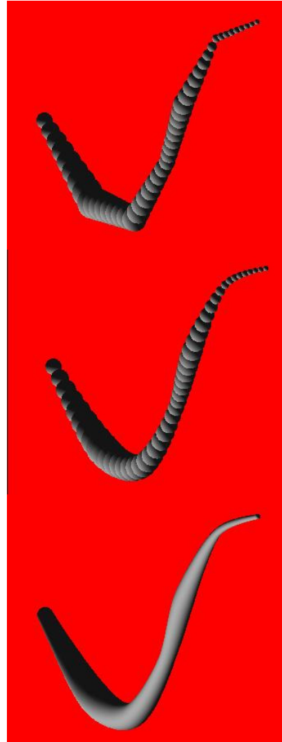
Fig.4. (Top) Linear subdivision gives us a string of pearls which resemble a set of connected cones. (Middle) 4-Point subdivision more accurately captures the curvature of the original string. (Bottom) Both of these approaches still result in “ridges” between the pearls, which we seek to remove by further interpolating the radii of adjacent pearls to include the values within these ridges.
